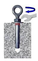
Tighten to recommended torque
