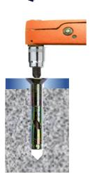
Tighten to recommended torque
