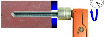
Drill correct diameter hole to correct depth
