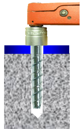
Tighten with torque wrench to recommended torque
