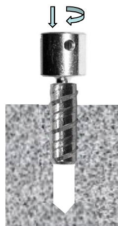
Insert anchor into concrete using suitable impact wrench
